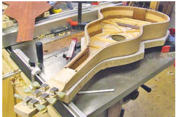
▲ Pic.17 Glue kerfed linings in place on front and back. The glued headstock aids alignment. Note the tail block and solid linings in the neck
